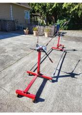
Auto body Rotisserie for Sale, Made from Two engine Stands, can be modified for any kind of restoration project. I built it for a Model T project. Comes with all the engine stand parts and the materials I used to modify it.
